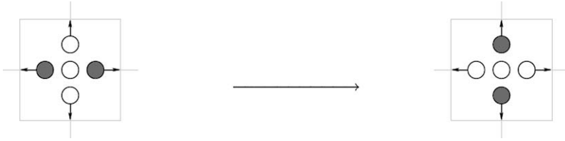
Figure 2 Example for interaction of particles at two-dimensional square lattice node r ; gray dots denote the presence of a particle in the respective channel. No confusion should arise by the arrows indicating channel directions.
